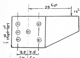
shear stress in the rivet is limited to 630 kg/cm 6 find the diameter of the rivets.
